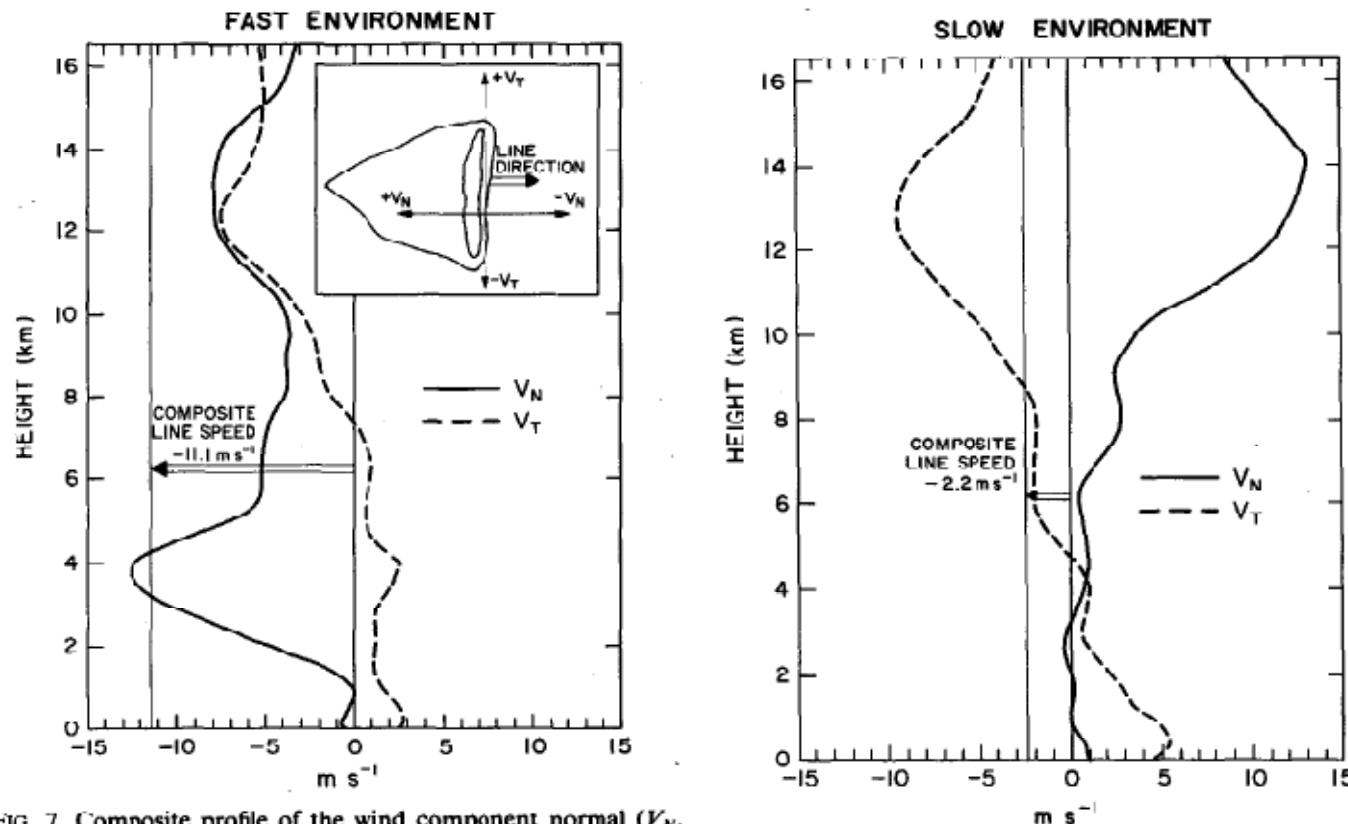
FIG. 7. Composite profile of the wind component normal ( $V_N$ , solid) and parallel ( $V_T$ , dashed) to the leading edge of a squall line for the environment. The mean line speed is shown by a thin vertical line.
